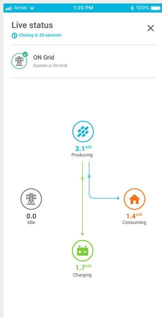
Solar production is powering the home and charging the batteries.
