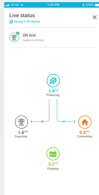
Solar production is powering the home, and because the batteries are fully charged, excess generation is exported to the grid.
